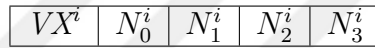
Figure 3.5: Tet20 structure. Each field is an integer and four bytes long. The tetrahedron data occupies 20 bytes of memory.
