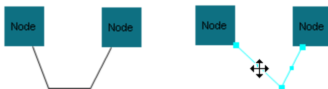
Figure 17 Bend point deletion; initially the edge has two bends (left); upon drag and release of the left bend, it is deleted to leave the edge with only one bend (right).
