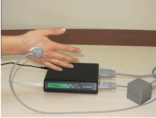
Fig. 2. The gesture recognition setup using a magnetic 3D position tracker.
