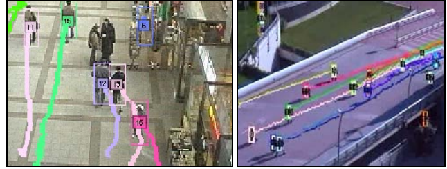
Figure 6: Fast kernel-based tracking of multiple targets using motion information.
