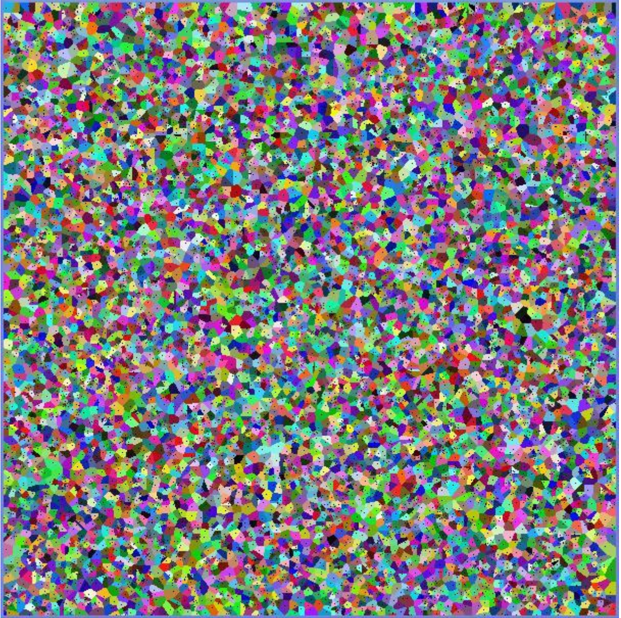
Figure-16: Ordinary Voronoi Diagram of 10000 randomized point sites Error Threshold: 1 Resolution: 600x600 Response Time: 20.218 Seconds
