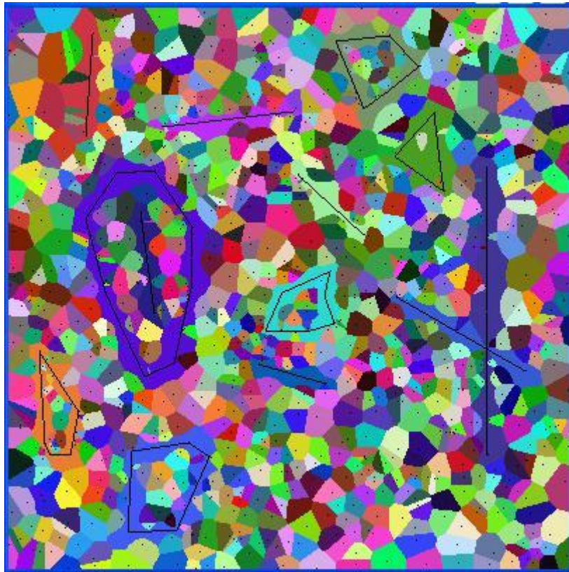
Figure-20: Generalized Voronoi Diagram of 6 polygon sites, 7 line sites and 1000 randomized point sites Error Threshold: 1 Resolution: 400x400 Response Time: 1.063 Seconds
