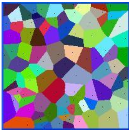
Figure-19: Ordinary Voronoi Diagram of 100 randomized point sites Error Threshold: 50 Resolution: 200x200 Response Time: 0.015 Seconds
