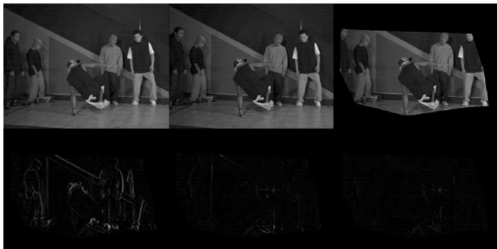
Fig. 3. Experimental results for Breakdancers . Left, top row (left to right): reference, target, and predicted images. Left, bottom row (left to right): prediction error at the beginning, before nonlinear optimization, and after nonlinear optimization. Right: representation quality versus # vertices.
