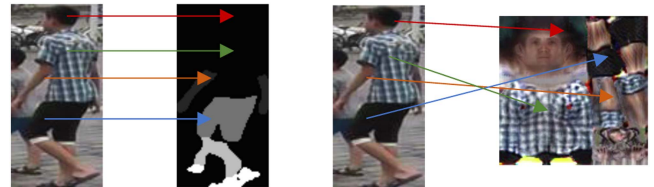
Fig. 1. Texture estimation is not aligned, unlike many tasks with input-output alignment (e.g., part segmentation).
